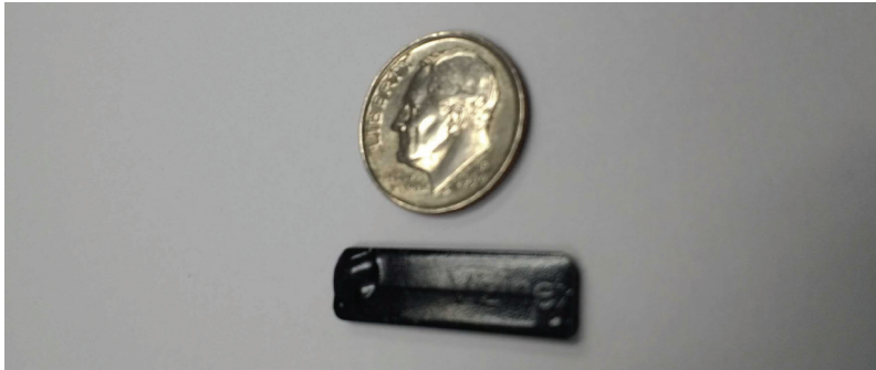
A small footprint, low profile mount-on-metal tag.
