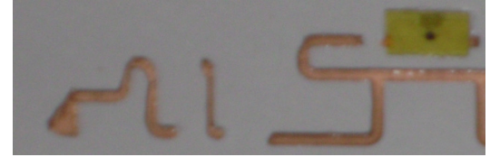
RCDSecure™-enabled windshiled tag that has self-destructed from being removed from a windshield; Antenna detachment renders the tag useless.
