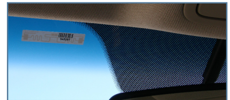
RCD Windshield tag on glass behind the rear view mirror, with RFID antenna visible.
